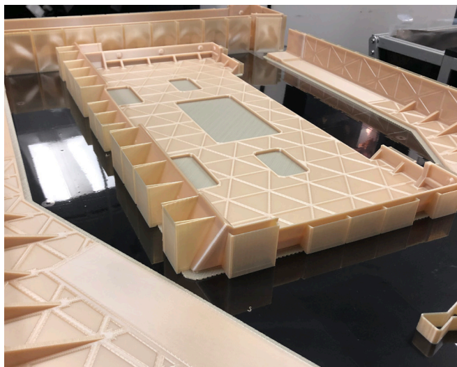
These 3D printed parts replace assemblies that were previously made using a more resource-intensive composite laminate process.
